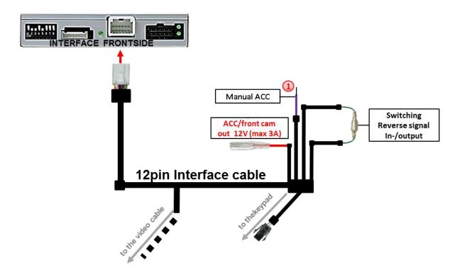
Connect the purple coloured wire Manual ACC of the 12pin interface cable to S-contact terminal 86s +12V (e.g. glove compartment illumination).
