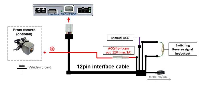
The red power supply output ACC/front cam out 12V (max 3A) can be used to power a front camera. If Dip 1 is set to ON (of the black 8 dips), the power supply output gives +12V (max 3A) when reverse gear is engaged incl. 10 seconds delay after reverse gear is disengaged.
