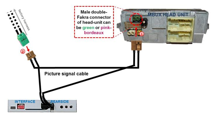
Connect the female Double-Fakra connector of the picture signal cable to the head unit's green or pink-bordeaux coloured Double-Fakra connector.
