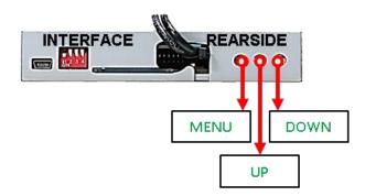
The picture settings are adjustable by the 3 push-buttons at the rear-side of the video-interface. Press the MENU button to open the OSD settings menu or to switch to the next menu item. Press UP and DOWN to change the selected value. The buttons are placed inside in the housing to avoid accidental changes during or after the installation. Picture settings must be done separately for all video inpouts while the corresponding input is selected and visible on the monitor.
