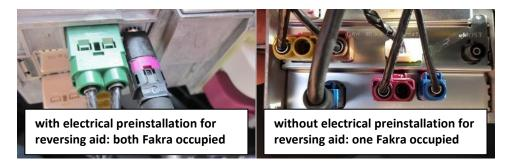
2 Connect the green or pink-bordeaux coloured female Double-Fakra connector of the vehicle harness to the picture signal cable's Double-Fakra connector.
